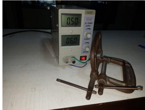
Figure 8.1 Setup for measurement of armature resistance
