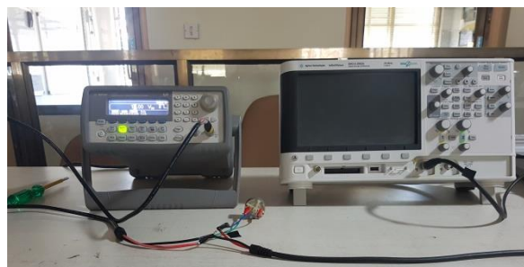
Figure 8.3 Setup for measurement of inductance
